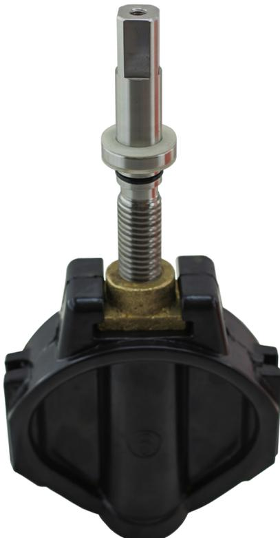
As standard all Series GVI Gate Valves feature a one-piece forged shaft with an integral thrust collar supported in both directions by replaceable permanently lubricated thrust bearings. The one-piece shaft eliminates the seal damage and leakage that often occurs with gate valves that utilize a split ring collar to retain thrust. Shafts are stainless as standard, with many options available to meet project requirements.
